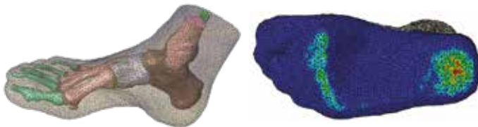
3D mesh of foot and simulated plantar pressure in Abaqus
